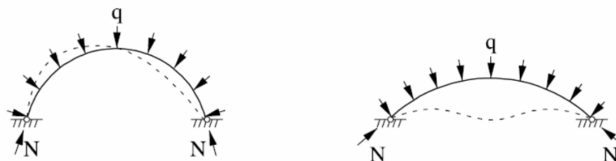
(a) Anti-symmetric bifurcation buckling (b) Symmetric snap-through buckling
