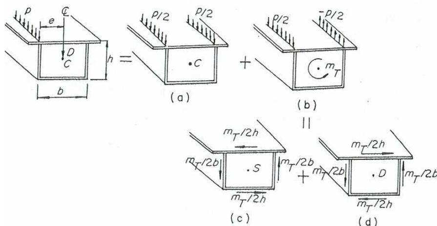
Figure 3. Decomposing the load into symmetric and anti symmetric loading
