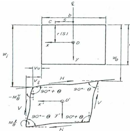
Figure 4. Distortion of the Rectangular Box section
