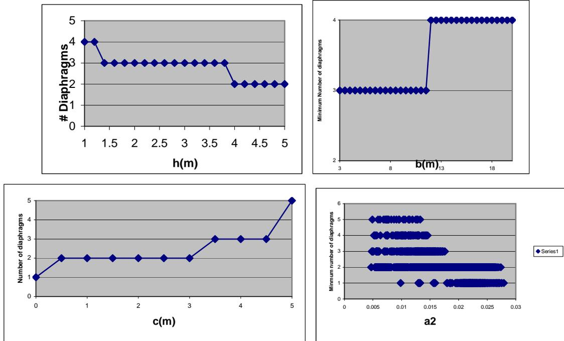
Figure 7. Variation of Number of Diaphragms with Key Parameters
