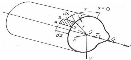
Figure 2 Generalized Section under Torsion
