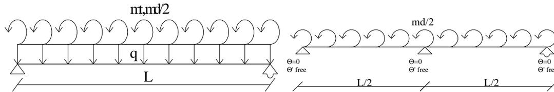
Figure 6. Simply Supported Beam without and with Intermediate Diaphragm
