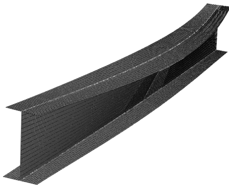
Fig. 2: Lowest buckling mode shape for IPE 300 ( L=3000\text{mm} )
