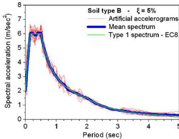
Fig. 3: Response spectra of the examined earthquakes
