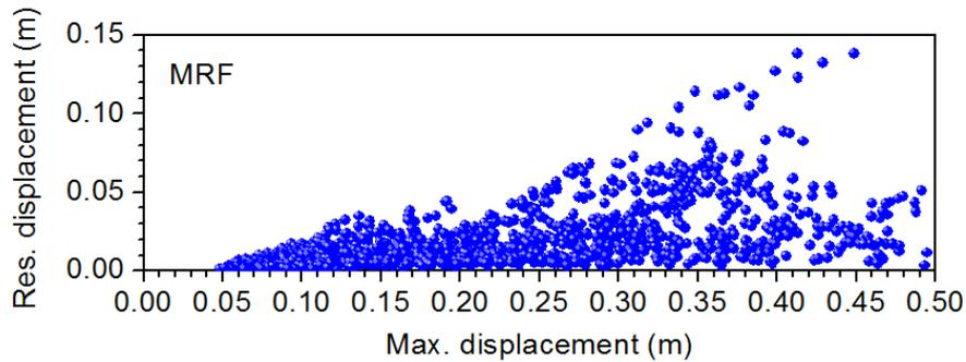
*Fig. 4: Permanent deformation - maximum displacement diagram for the examined MRF*
