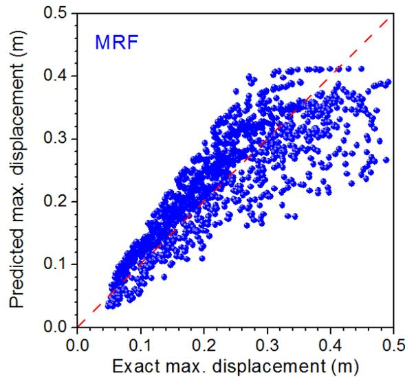
*Fig. 6: Evaluation of maximum displacements for the examined MRF*
