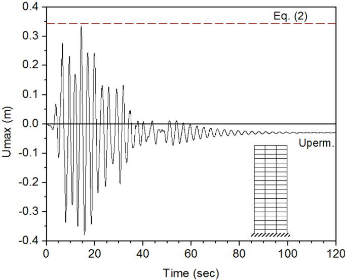
*Fig. 8. Displacement time history for a typical MRF*
