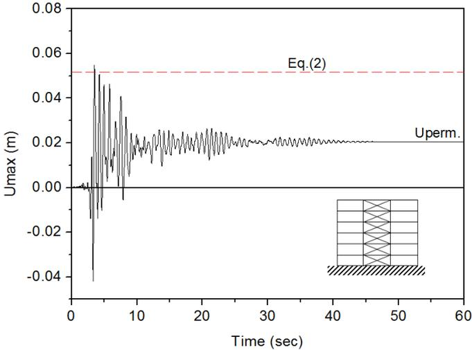
*Fig. 9. Displacement time history for a typical CBF*
