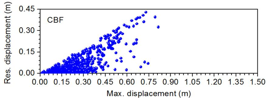
*Fig. 5 Permanent deformation - maximum displacement diagram for the examined CBF*
