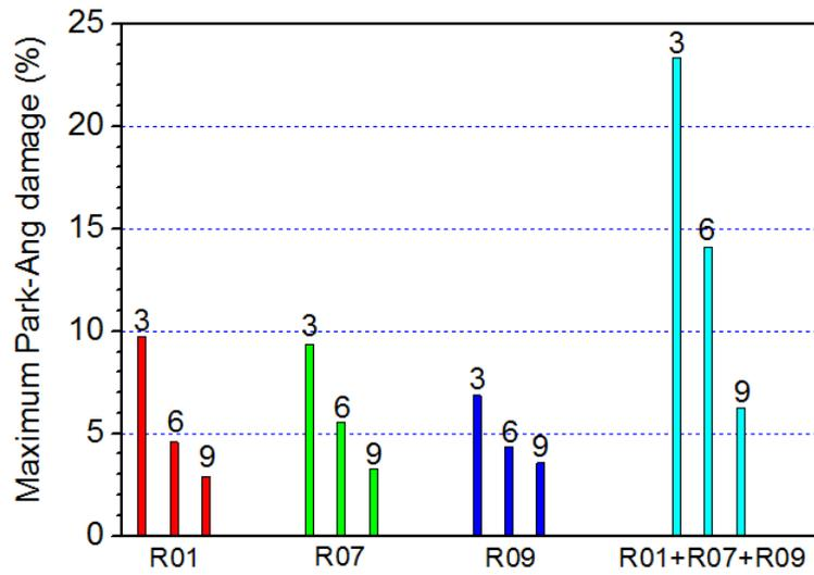
*Fig. 2. Maximum local damage for a 3-, 6- and 9-storey CBF*
