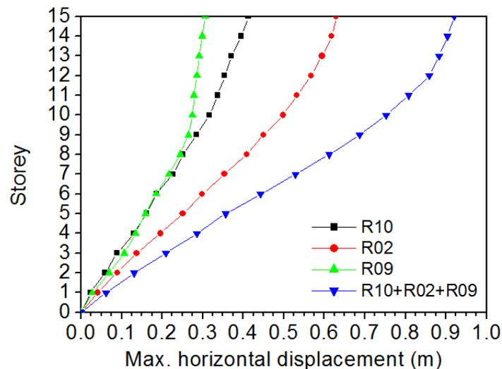
*Fig. 3. Maximum hor. displacements for a 3-storey MRF under the Imperial Valley (1979)*
