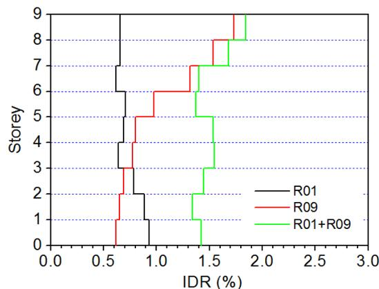
*Fig. 1. IDR distribution for a 9-storey CBF under the R01 and R09 records*
