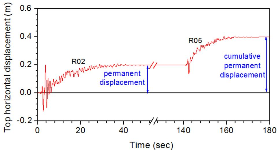
*Fig. 4.* Displacement time history for a 12-storey CBF under the R02-R05 sequence
