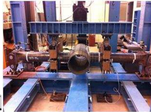
Fig.1. Specimen geometry for the OPB tests.
