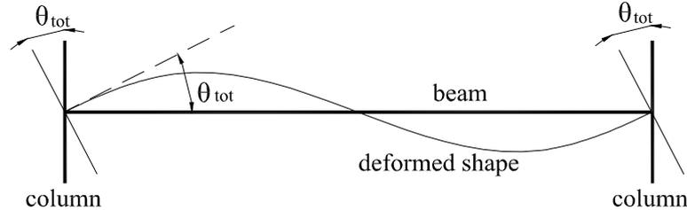
Fig. 3: The induced rotation at the beam ends.
