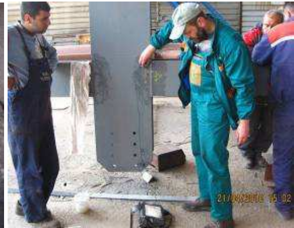
Fig. 19 "UT" test of welding
