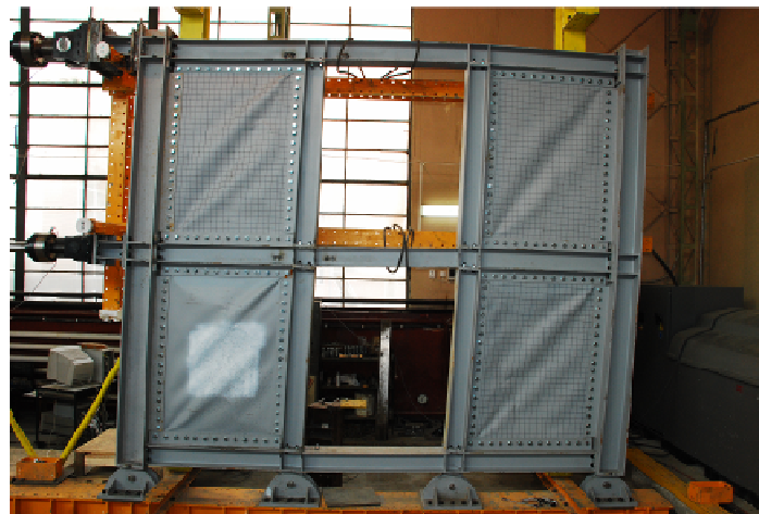
Fig.6 Deformed shape after the test
