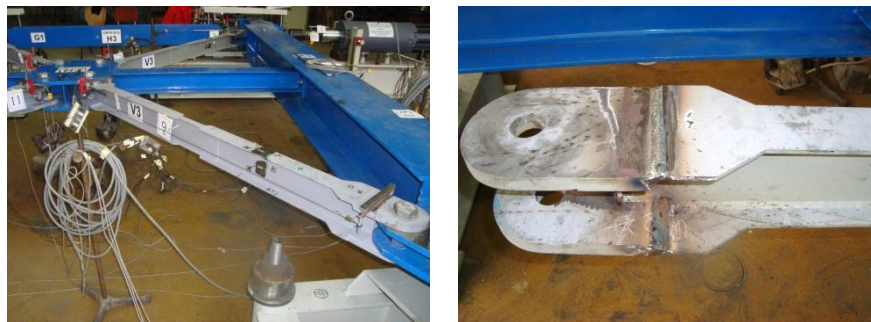
Fig. 3 - General view of the proposed solution. Frame configuration - left. Connection solution with two gusset plates and two fitted bolts – right.
