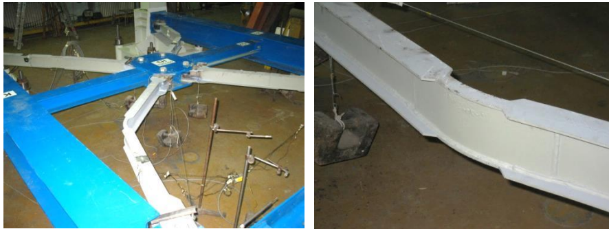
Fig. 10 - Buckling of compressed diagonal (left); MCS of buckled diagonal (right)
