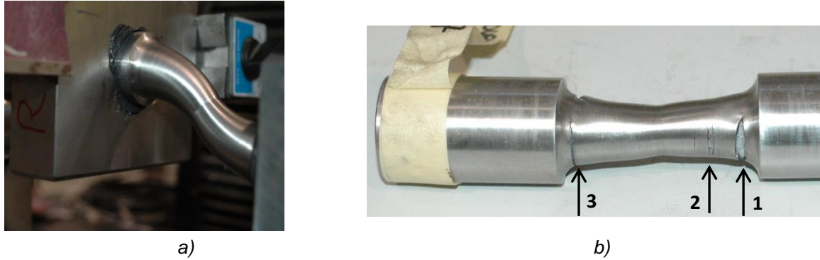
Fig. 5. a) Large displacement of the SS-WHP2 specimen under monotonic loading; b) fracture (typical) of a WHP under cyclic loading
