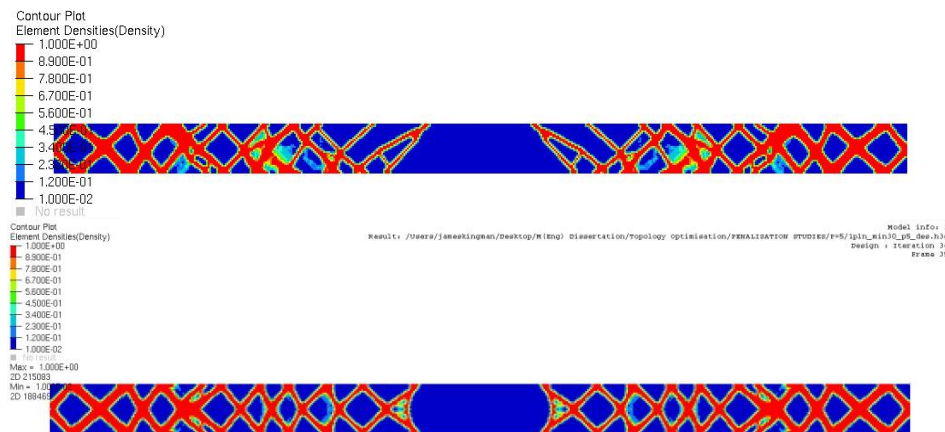
Fig. 4: (a) Results of a topology optimisation study on a beam web, (b) Results of a topology optimisation study on a beam web incorporating a symmetry constraint
