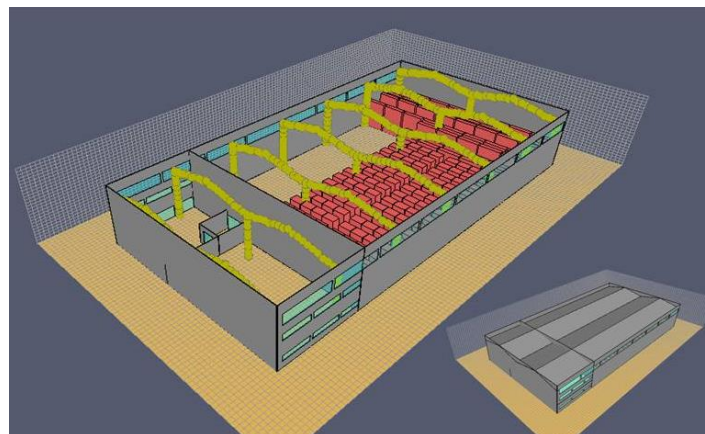
Fig. 2 3-D model of building and rectilinear grid for CFD analysis
