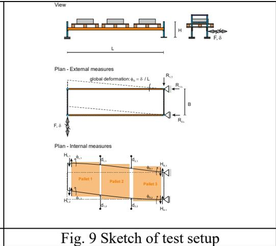
Fig. 9 Sketch of test setup
