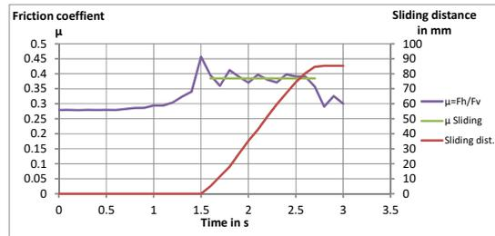
Fig. 6 Example for derivation of friction coefficients from tests
