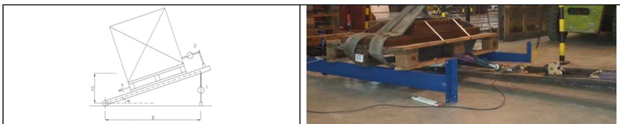
Fig. 5 Setup of frictions tests (left: FEM tests; right: performed tests)
