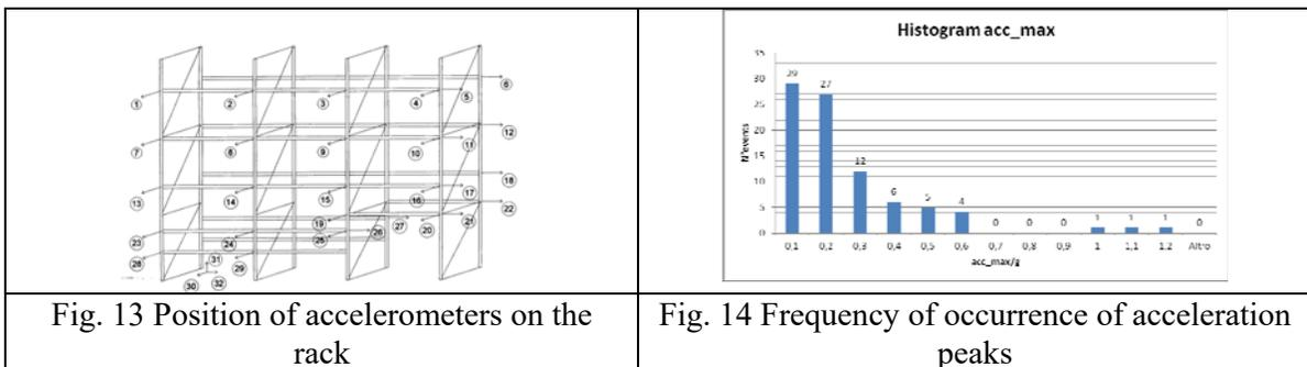
For each event, by re-analyzing the acceleration time histories, indications were also derived on the deformation of the structure under impact loading due to the S/R actions, and its modal shapes.
