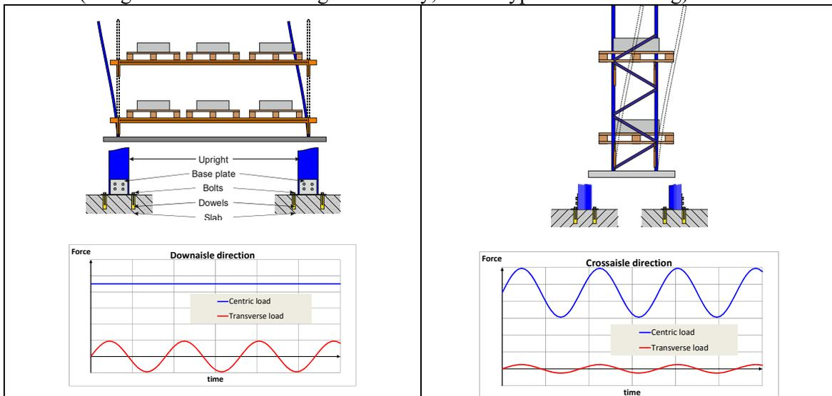
Fig. 12: Directions of rotation and loads on the base plate connection
