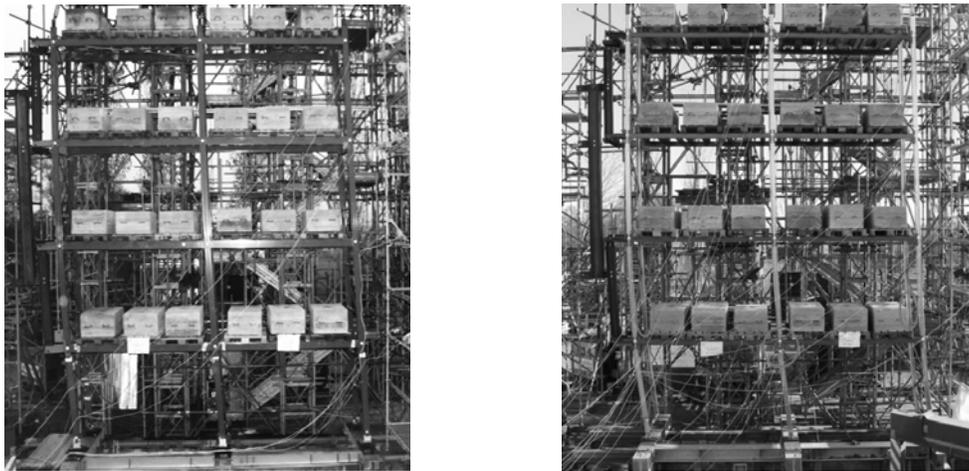
Figure 16 Deformed shapes at the last loading increment of IP A (left) and IP C (right) structures
