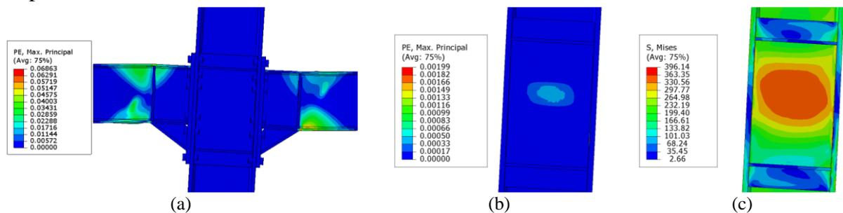
*Fig. 10: Parametric numerical simulations. a) plastic strain in joint, (b) plastic strain in panel zone, (c) Mises stress in panel zone at ultimate strength of the joint*
