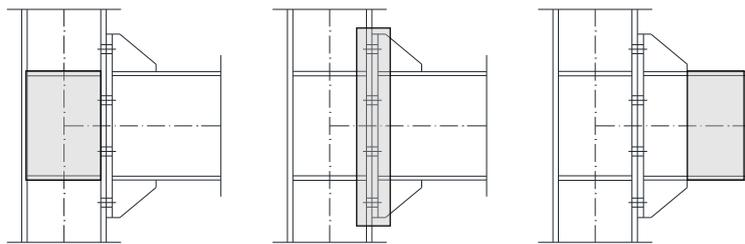
*Fig. 3: Plastic regions of the joints: a) web panel, b) connection and c) beam.*
