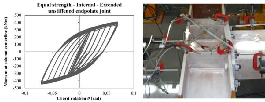
Fig. 6: Moment-rotation behaviour of extended unstiffened end-plate equal strength joint tested in UNINA lab: plastic deformation contemporarily occurring in column web panel zone, connection zone and beam flange.
