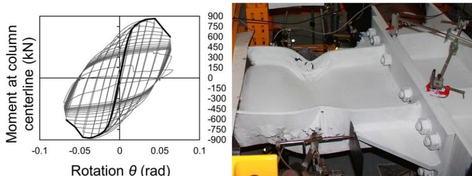
*Fig. 4: Moment-rotation behaviour of equal strength stiffened extended endplate joint tested in UNINA lab: plastic deformation contemporarily occurring in connection zone and beam flange.*
