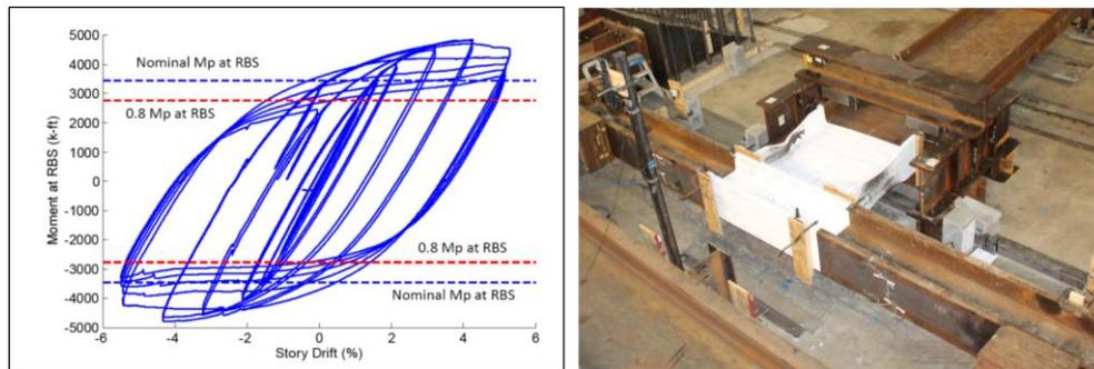
Fig. 7: Moment-rotation behaviour of dog-bone joint tested in Virginia Tech lab: plastic deformation contemporarily occurring in the reduced beam zone.
