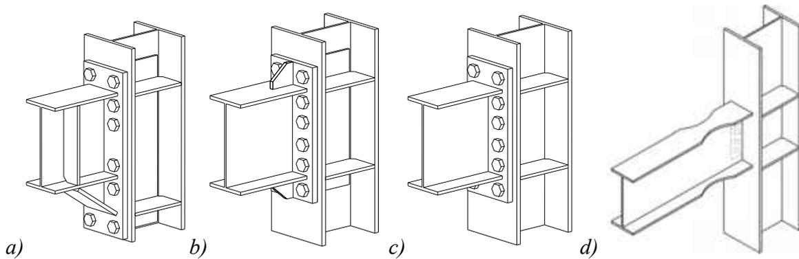
Fig. 1: Beam-to-column joints investigated in the framework of EQUALJOINTS project: a) Bolted haunched joints b) Bolted extended stiffened endplate joint c) Bolted extended unstiffened endplate joint d) Welded dog-bone joint
