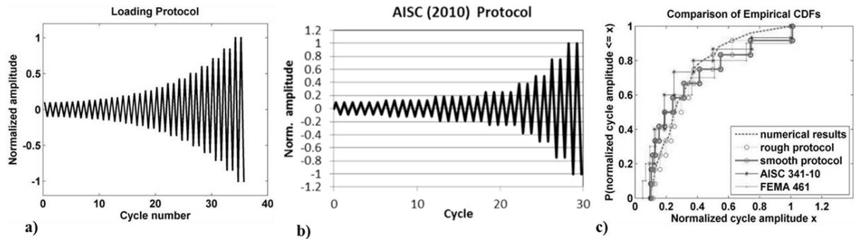
Fig. 9: Derived loading protocol (a) AISC 2010 loading protocol (b) comparison of CDF (c)
