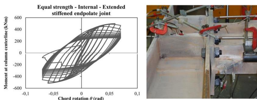
*Fig. 5: Moment-rotation behaviour of equal strength extended stiffened end-plate joint tested in UNINA lab: plastic deformation contemporarily occurring in connection zone and beam flange.*
