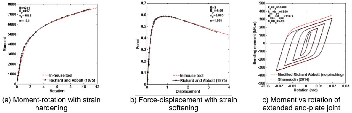
Fig. 8: Developed Modified Richard Abbott model vs. experimental results.
