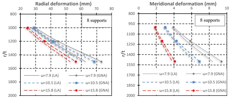
Figure 5: Radial and meridional deformations in the case of 8 supports, varying  $r/t$  ratio and panel height  $\omega$ .
