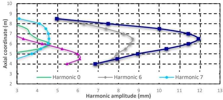
Figure 2: Amplitude of the harmonic terms along the meridian of Silo A.
