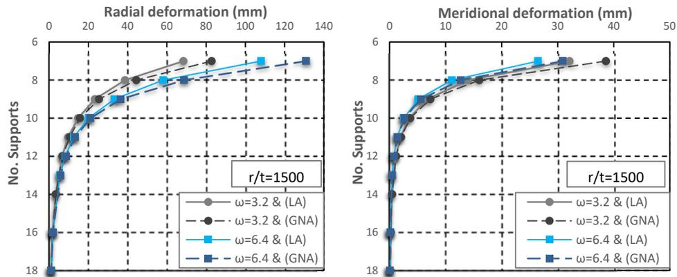
Figure 6: Radial and meridional deformations in the case of  $r/t$  ratio = 1500, varying no. of supports and panel height  $\omega$ .
