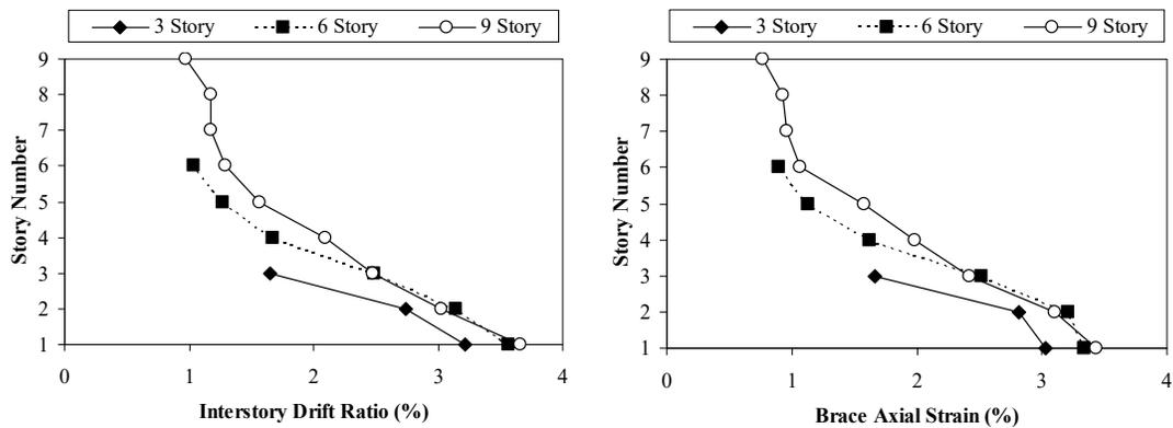
Fig. 3: Interstory drift ratio and brace axial strain of archetypes
