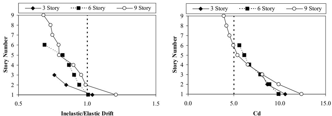
Fig. 4: Ratio of inelastic and elastic drift and variation of deflection amplification factor
