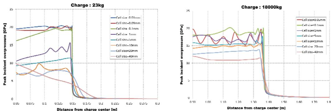
Fig. 3: Incident overpressure distribution when the shock front reaches the face of the 23kg [left] and 18000kg [right] charge
