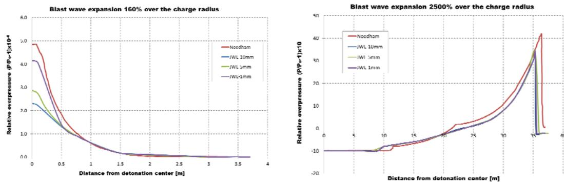
Fig. 1: Relative overpressure values at 0.58ms [left], and at 27.20ms after detonation [right]
