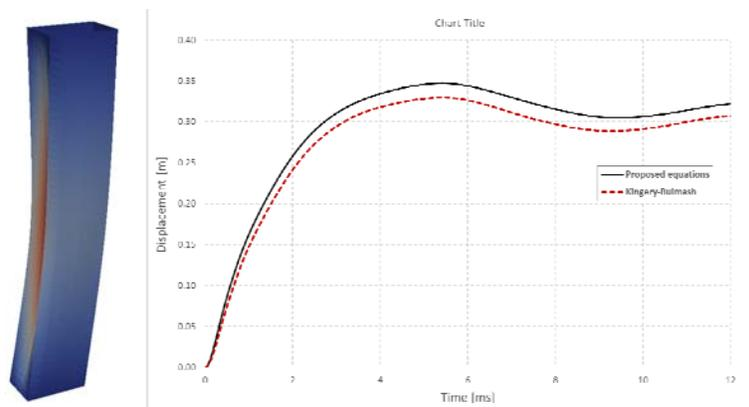
Fig. 5: Displacements at mid-span of beam section
