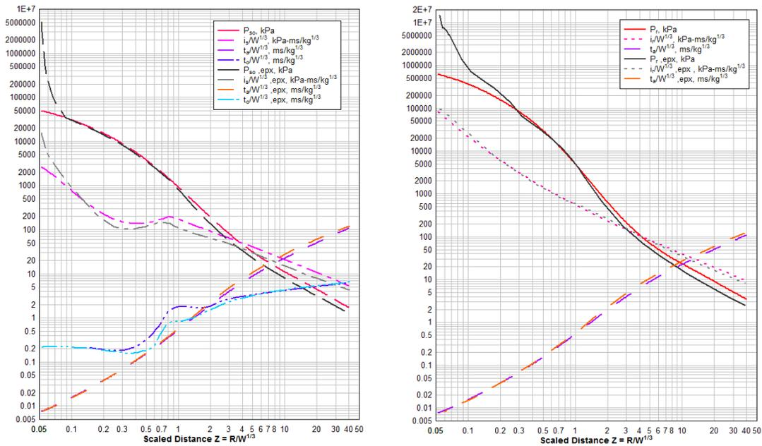
Fig. 4: Additional incident [left] and reflected [right] parameter curves of positive phase of shock spherical wave of TNT charges from free-air bursts
