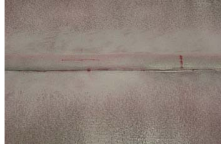
Fig. 1. Two linear indications detected by dye penetrant testing.
