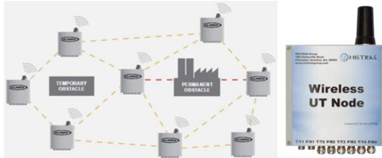
Fig. 1: Wireless Mesh (left) and wireless UT node (right).
